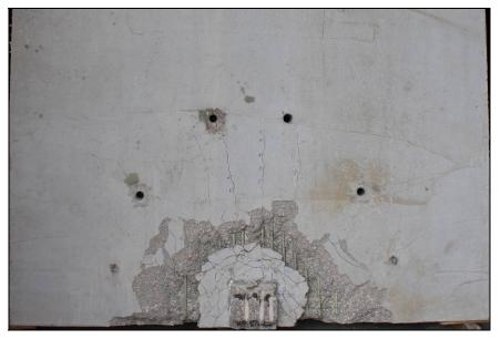
Figure 5. Cracking pattern at failure for connection E60.
