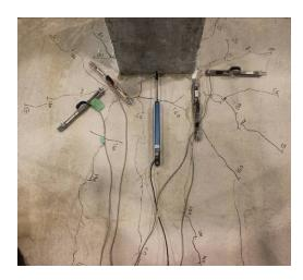
a) b) Figure 4. Cracking pattern after the application of gravity load: (a) connection E50, (b) connection E60.
