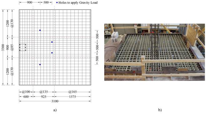
Figure 1. Typical details of test connections (dimensions in mm): (a) top reinforcement mesh layout, (b) reinforcement configuration.
